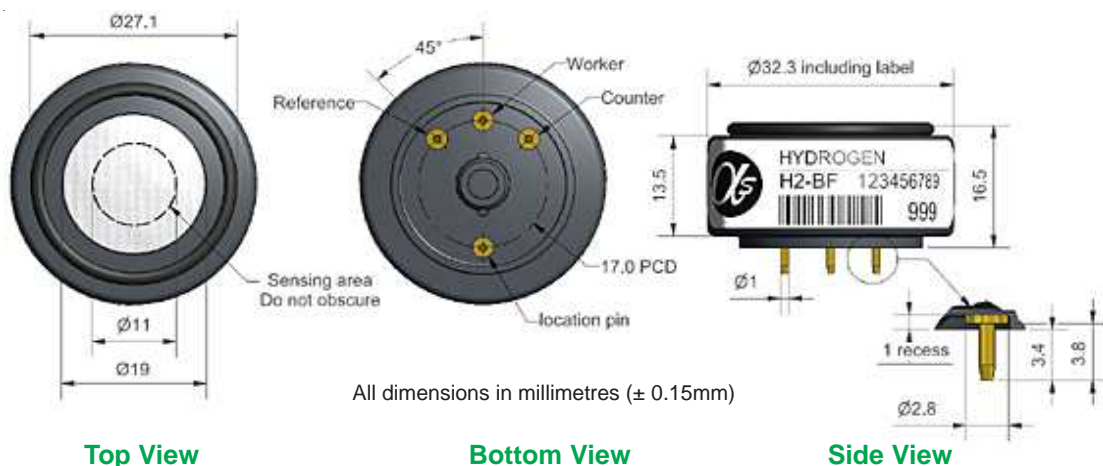
Figure 1 H2-BF Schematic Diagram
